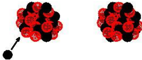
Before collision of neutron (black) with chlorine-35 nucleus, 17 protons (red) and 18 neutrons. After collision, neutron is captured, resulting in chlorine-36 with 17 protons and 19 neutrons.
